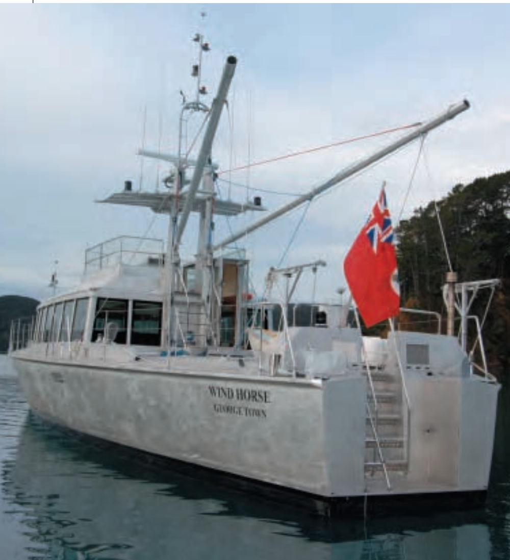
Details of the boat's stern. Notice the simplicity of boarding at the stern, as well as the high quality of the unpainted metalwork.
