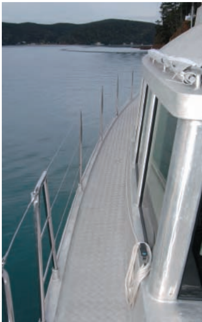
Left: Side decks are wide and well secured, with handholds everywhere. The tread pattern of the aluminum plate used on deck provides an added measure of safety. Right: View aft from the foredeck. Visibility is terrific from this utilitarian flybridge, and clean, uncluttered decks keep the boat simple and low profile.
