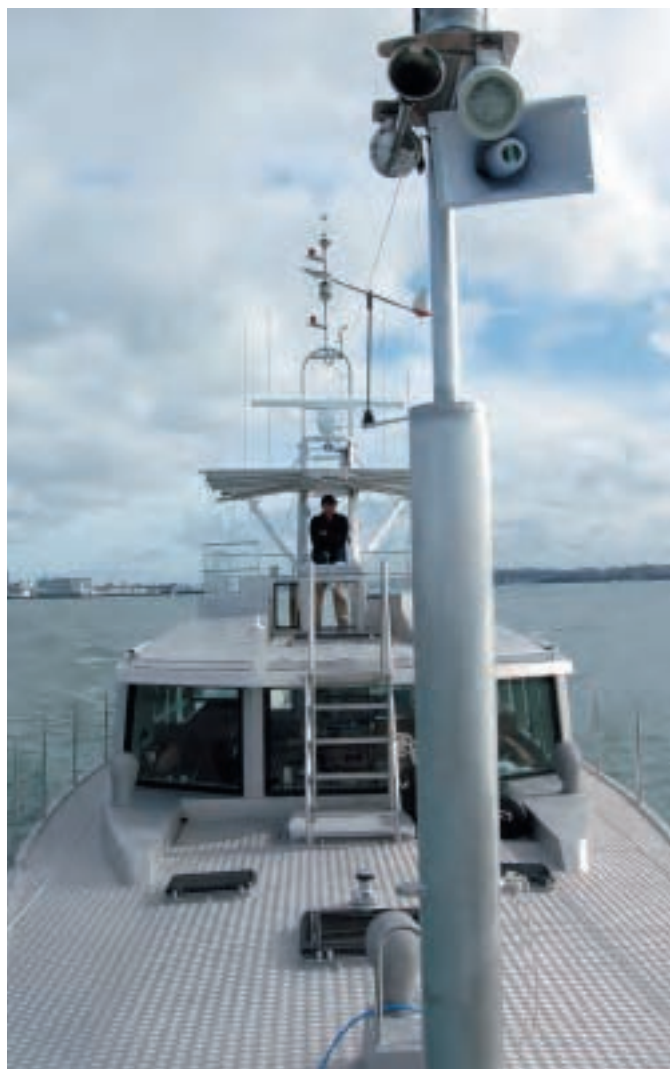
Left: Side decks are wide and well secured, with handholds everywhere. The tread pattern of the aluminum plate used on deck provides an added measure of safety. Right: View aft from the foredeck. Visibility is terrific from this utilitarian flybridge, and clean, uncluttered decks keep the boat simple and low profile.
