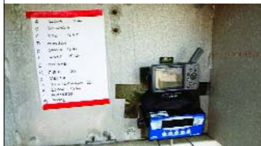
The strain gauge (inset) fed the data directly into the computer as well as to a second read-out on deck (below)
